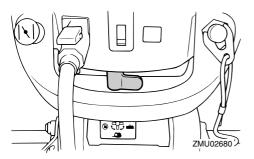
If you are using an external fuel tank, connect the fuel joints securely and squeeze the primer pump with the outlet end up until you feel it become firm (if equipped the fuel joint).
